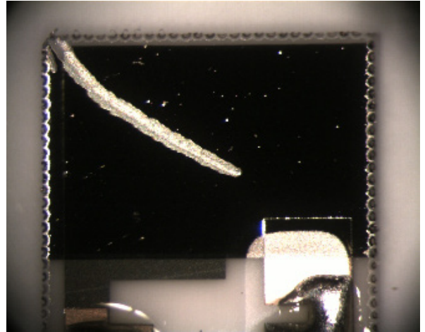
Picture 8: Sensor with a scratch
