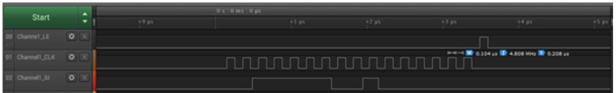
Figure 11 – Scope Capture of SAM signals for Writing to an Attenuator
