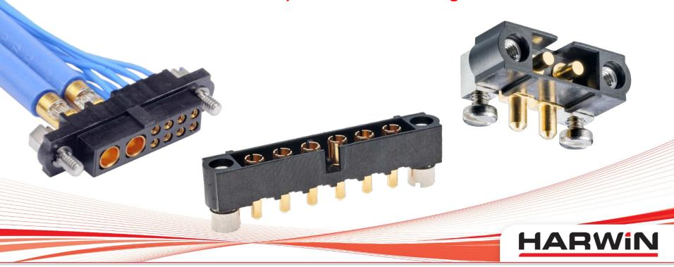
Mix-Tek uses the same outer housing design as J-Tek, with each power contact taking up the space of 4 signal contacts (giving 4mm pitch). The original power contacts are capable of up to 20A, and the latest High Power contacts will carry 40A each.
