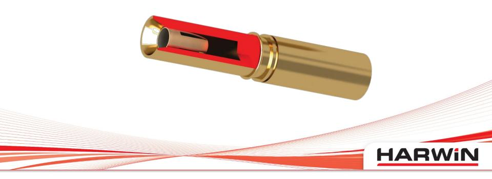
A 4-fingered Beryllium Copper female contact gives superb performance, for both electrical and mechanical specifications. This inner "contact clip" is stamped and plated with a durable gold finish at our UK headquarters. The spring performance of the contact gives the environmental resistance to shock and vibration, with a temperature range up to 125 degrees C.
