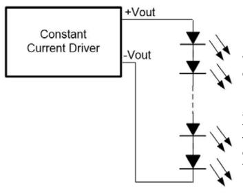
With this configuration a single constant current driver illuminates the entire string of LEDs.
