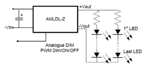
If any LED fails open all LEDs in that string will stop operating, while the other strings will continue operating. If any LED fails short, that string will carry higher current that the other strings increasing the stress levels of the remaining LEDs.
