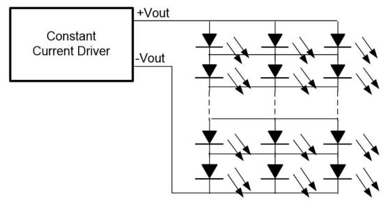
A matrix configuration is similar to a parallel configuration but extra connections are used to help minimize the effects of individual LED failures. Multiple LEDs are connected in parallel and then stacked is series. The total voltage and current would remain unchanged from the parallel configuration. If any LED fails short would cause the row of LED to stop operating while the remaining LEDs would be unaffected. Current sharing is a directly related to the matching of the LEDs.
