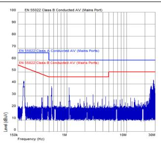
in combination with PKM 4817NH  $V_l = 53 V, C_{01} = 330 \mu F$  electrolytic // 130  $\mu F$  ceramic,  $I_{01} \approx 17 A$  $(I_{0\_DCDC} \approx 75 A), I_{02} = 3.6 A$
