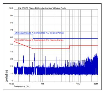
in combination with 2 x BMR 456 0004  $V_l = 48$  V,  $C_{01} = 470 \ \mu\text{F}$  electrolytic // 30  $\mu\text{F}$  ceramic,  $I_{01} \approx 17 \text{ A}$ ( $I_{0 \ DC/DC} = 2 \times 32 \text{ A}$ ),  $I_{02} = 3.6 \text{ A}$
