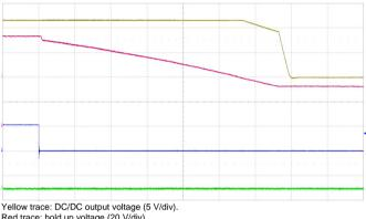
Red trace: hold up voltage (20 V/div) Blue trace: input voltage (50 V/div). Green trace: Power Good (5 V/div). Time scale: (2 ms/div). Shutdown with default configuration for Power Good.
