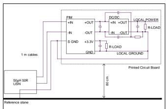
Conducted EMI Test set-up.
