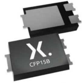
CFP15B (SOT1289B) 5.8 x 4.3 x 0.95 mm* R_{th(j-sp)} = 7 \text{ K/W}
