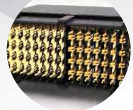
Ultra-high density; single-ended or differential pair wafers
