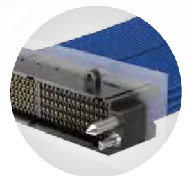
IN DEVELOPMENT: Flyover® cable assembly for extended signal reach
