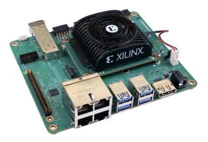
To aid development of robotic solutions, AMD Xilinx also offers the Kria™ KR260 Robotics Starter Kit, which provides not only the Kria K26 SOM, but also a carrier card that contains many standard interfaces used in the development of robotic systems. The Kria Robotics Starter Kit therefore enables development of robotic applications while custom carrier cards are being developed, reducing development timescales and technical risk.
