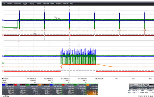
Figure 89 – 265 VAC, 50 Hz. Ch1: I DS , 200 mA / div., 1 s / div. Ch2: 12 V I OUT , 1 A / div., 1 s / div. Ch3: V DS , 200 V / div., 1 s / div. Ch4: 12 V OUT , 5 V / div., 1 s / div. Zoom: 20 ms / div. Auto-restart ON Time: 45 ms. Auto-restart OFF Time: 1.64 s.
