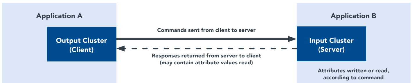
Figure 5.14. A Zigbee communication model
