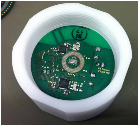
Figure 10.12. Wireless pressure sensor node
