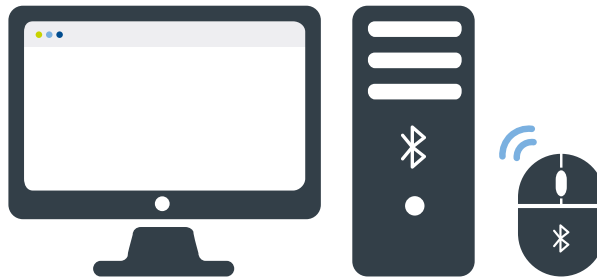
Figure 5.9. Bluetooth Low Energy peripheral and central devices
