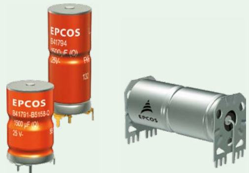
Figure 3. EPCOS aluminium electrolytic capacitors for automotive electronics are characterised by their extremely high vibration strength of up to 60g and maximum operating temperatures of up to 150°C.
