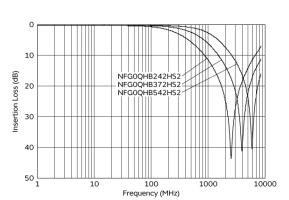
**Common Mode Insertion Loss Characteristic** (Main Items)(Typical Value)
