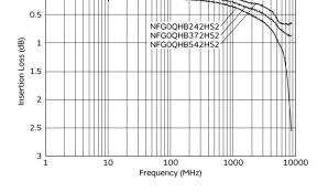
**Differential Mode Transmission Characteristics** (Typical Value)
