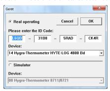
Now for the "Device", select the device driver "14 Hygro-Thermometer HYTE-LOG 4800 Bd". The activation code will be registered automatically. Confirm the dialogue with ,OK'. Now open the option "Extras" in the menu and then go to the sub-menu "Interface". Put in the corresponding interface.
