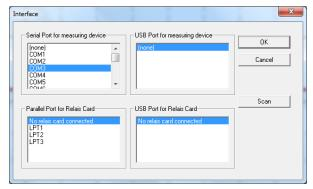
The user interface – if not known – can be determined in the device manager under Windows. (Control panel P System P Hardware P Device Manager P Connections) The PCLOG start screen appears. The measured values of the sensors are displayed on the left side.
