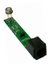
Place the sensor as described into the adapter board and then connect it with the help of the connection leads provided with the PC adapter. Then connect the PC adapter through the USB cable to the PC or your notebook.
