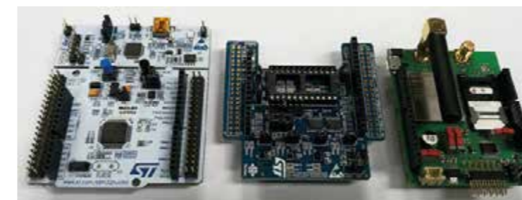
The Avnet Silica NB-IoT Sensor Shield starter kit with X-Nucleo sensor board and STM32 Nucleo-64 processor board already has its own test cloud for evaluating connectivity.
