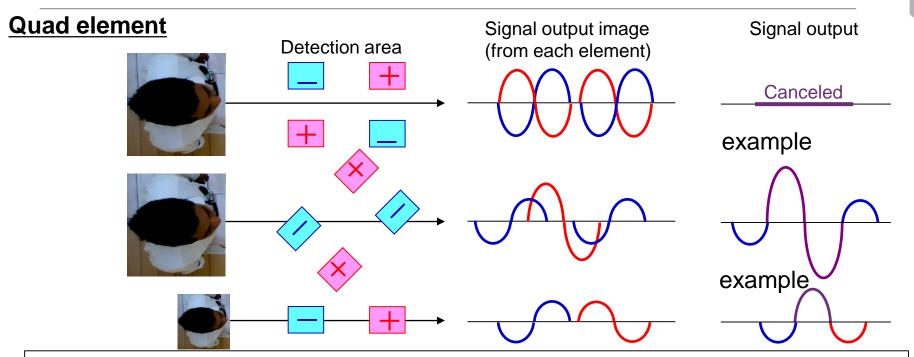
Quad element has the advantage in **the fine motion detection** when it is used in a ceiling mount detector. This performance comes from the arrangement of element polarity and number of detection area.
