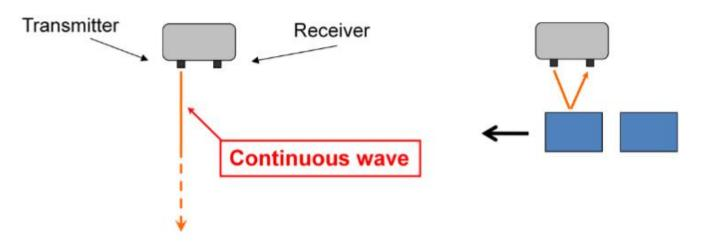
Received signal will not appear in the case that no object reflects the wave. Smaller distance between sensor and object make signal bigger.
