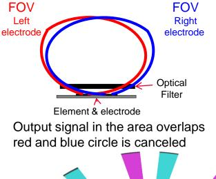
If an optical system is not used in front of sensor, directivity of the sensor is as shown in the left figure and the detection area is not formed.
