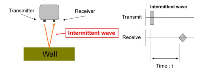
Measuring the time from transmitting to receiving (using clock) Time x Sonic speed(340m/s) = Distance to the object
