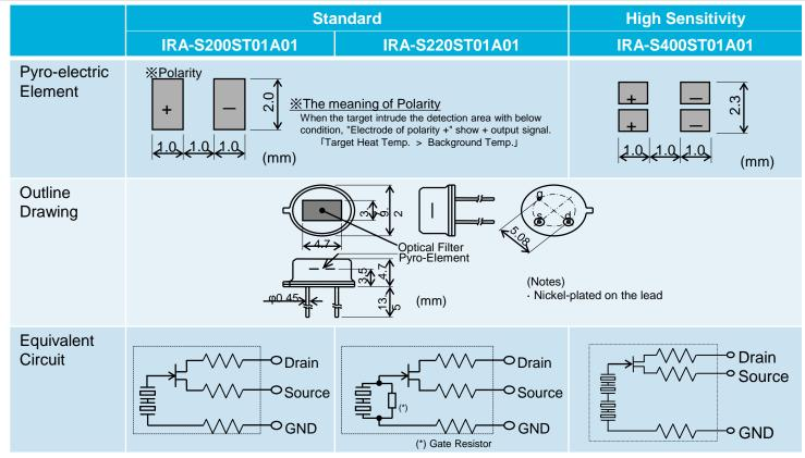
Rg (gate resistor) makes the temperature characteristics stable.
