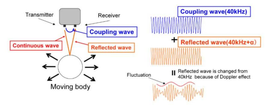
The movement is detected by fluctuations of mixed signal.
