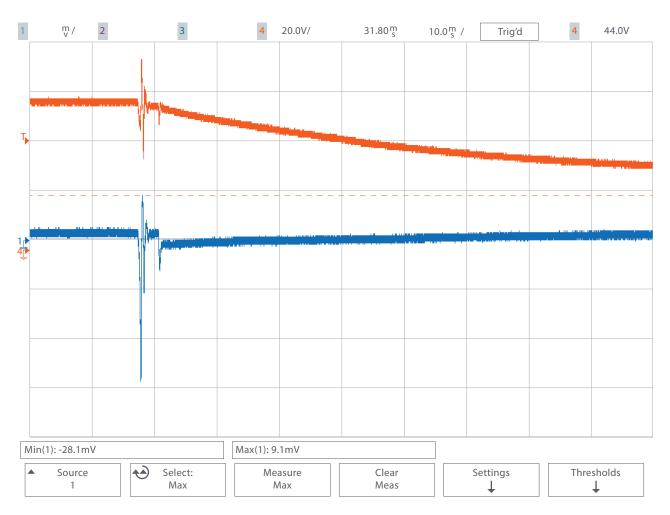
Channel1 (Red) above shows the resultant output voltage spike occurring when the negative current limit is reached, and the output stage goes high impedance. Energy from the load is no longer being dissipated by the power supply and the voltage rises.
