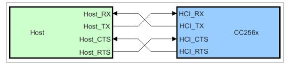
When the UART Rx buffer of the CC2564C passes the "flow control" threshold, it will set the UART\_RTS signal high to stop transmission from the host.
