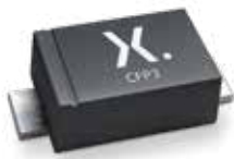
CFP3 (SOD123W) 2.6 x 1.7 x 1.0 mm* R_{th(j-sp)} = 18 \text{ K/W}
