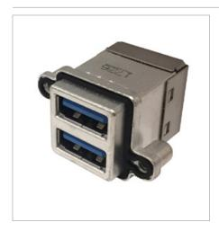
Amphenol's MUSBR series of ruggedised USB connectors with die cast housings and IP67 sealing is now available in 3.0 speed. The rugged series provides reliable performance in extreme conditions for the most demanding applications, and mates with standard USB plugs. The connectors are available in right angle or vertical styles and single port or stacked versions. They have an operating temperature range from -55°C to +105°C for extreme conditions and are RoHS compliant.
