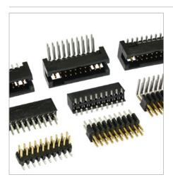
The Minitek127® 1.27mm connector system is an extensive range of modular connectors for all types of wire/cable-to-board applications. It includes straight and right angle, surface mount and through hole pin headers and board receptacles in different plating variations, as well as customised stacking headers, and an IDC version. The range is available in up to 100 positions.
