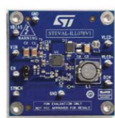
STEVAL-ILL078V1 1 A, up to 60V Vin, buck LED driver board based on the LED6000
