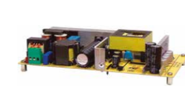
EVLCMB1-AIO210W 12 V - 210 W adapter based on TM PFC and HB LLC analog combo controller
