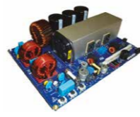
STEVAL-DPSTPFC1 3.6 kW PFC totem pole with digital inrush current limiter
