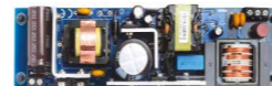
EVL80WLED-STCH03 80 W - 1 A primary side current loop control LED driver based on QR flyback converter
