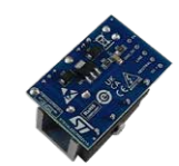
STEVAL-SCR002V1 Inrush current limiter for 1 kW AC/DC
