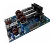
STDES-30KWVRECT 30 kW Vienna PFC rectifier reference design with digital control
