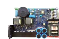
STEVAL-ISA147V3 500 W fully digital AC-DC power supply (D-SMPS)
