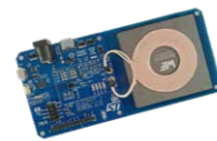
STEVAL-WBC86TX Qi wireless power transmitter for Baseline Power Profile (BPP) applications up to 5 W
