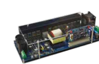
STEVAL-DPSLLCK1 3 kW Full Bridge LLC resonant digital power supply
