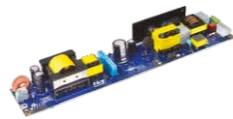
STEVAL-ILL066V2 100 W LED street lighting with DALI2.0 communication interface using the STLUX385A digital controller
