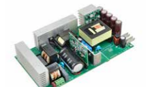
EVL400W-80PL 12 V - 400 W adapter based on CCM-PFC and HB LLC analog controller
