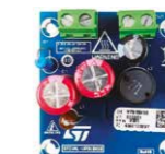
STEVAL-VP319X1B 5 V/600 mA buck converter
