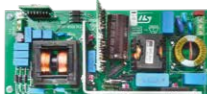
EVL6699-HVSL 150 V - 1 A LED driver featuring TM PFC and LLC resonant converter with L6699
