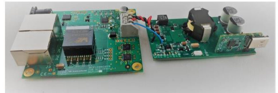
Connected to the NCP1096GEVB POE PD Demo
