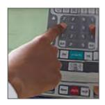
Capacitive Switch (recognizes when a conductive object, such as a finger, enters the field)
