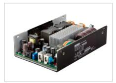
The PQU650 Series products are rated at 650W employing a `U' channel construction to operate with natural convection or forced airflow. The PQU650 series is a 1524 x 1016mm format capable of providing a continuous 650W output, with a constant current overload characteristic, and 800W "power boost" at output start to deliver transient loads.
