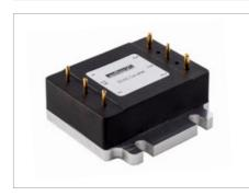
Murata's IRS Q48 & Q12 range offer an isolated single o/p, with 2250V isolation. The IRS range offers o/ps 3.3V, 5V, 12V, 15V & 24V variants. Two universal i/p ranges either 9V–36V or 18V–75V, allow for operation from 12V, 24V & 48V battery systems, Including meeting the requirements of EN50155.
