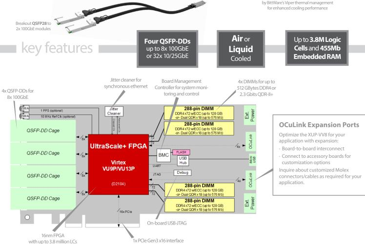
Module connects to one of the QSFP-DD cages on XUP-VV8
